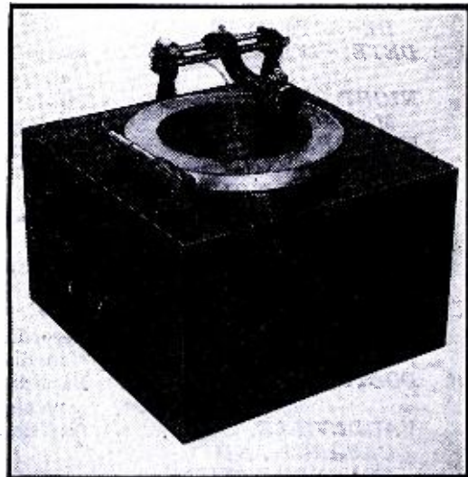
Duplex model A-16 Recorder and Playback instrument; provides for attachment for converting silent movies into home-talkies. A feature of this instrument is the use of a 2-speed gear drive which is said to permit piano recordings at 33 1/3 r.p.m. "absolutely free of wows." Magnetic cutter, crystal pickup. The wow-free operation of the driving mechanism is due to a unique arrangement of gears coupled directly to the turntable through an intermediate filter. The A-16 will cut 16-inch ungrooved blanks at 78 or 33 1/3 r.p.m. A flexible shaft, attached to an independent gear-train driven by the same motor, enables hand-crank 16-mm. movie cameras to be operated at either 16 or 24 frames per second for synchronized sound. A clutch disengages the camera drive when desirable.
