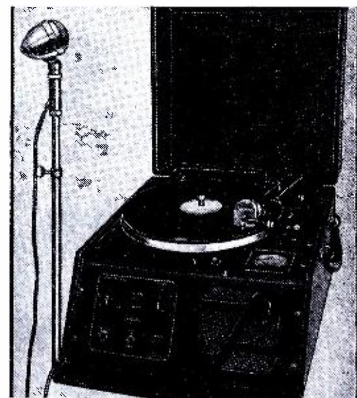
An "eye" tube is incorporated in the above-illustrated Wilcox-Gay "all crystal" model A-72 Recordio instrument for indicating correct recording level. The eye tube has a circuit network which creates quick response and slow recovery so that the indications will not confuse the lay operator. The output of this instrument with minimum distortion is 3 W.; "its response characteristic on microphone recording is acceptable from 50 cycles to 7,000 cycles," the manufacturer states. Rotary switch selects positions as follows: recording, transcription, public address. Cutter, pickup, and microphone, all are crystal.
